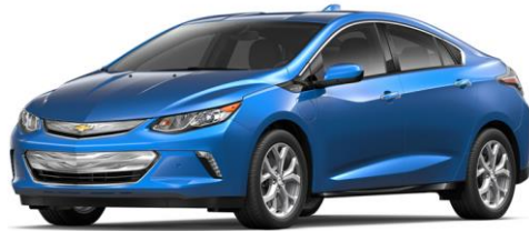
Chevrolet Volt, Series Hybrid with electric range of 50 miles
