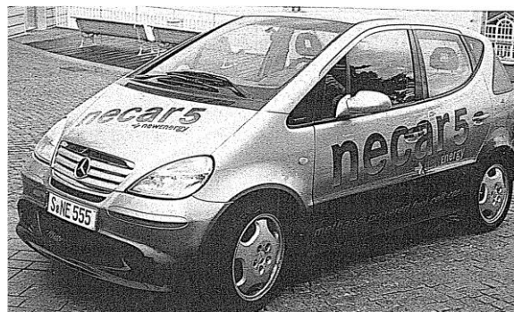
Fuel Cell vehicle, 400km range, 150km/h top speed
