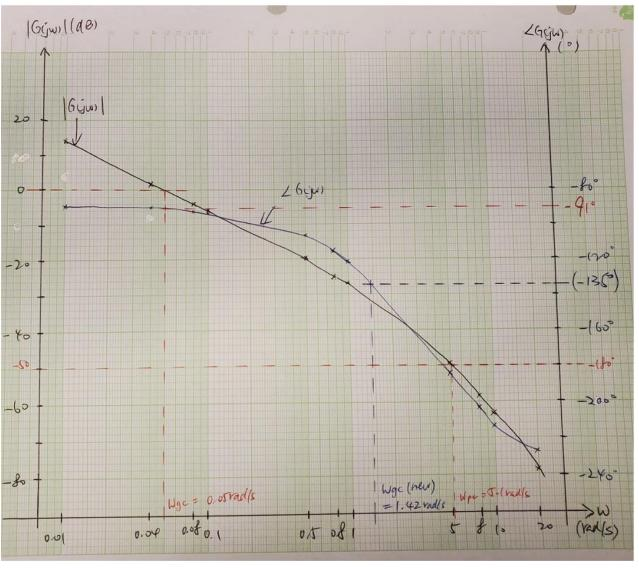
From the exact bode diagrams, the gain margin = 50 dB (G.M. =  $0 - |G(j\omega)|$ ) at 5.1 rad/s. Phase margin =  $89^{\circ}$  at 0.05 rad/s.
