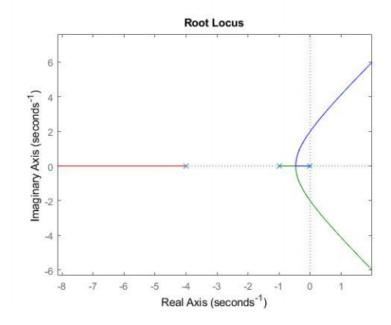
(b) The addition of zeros has the effect of pulling the root locus to the left, tending to make the system more stable. The root locus plot is shown below.
