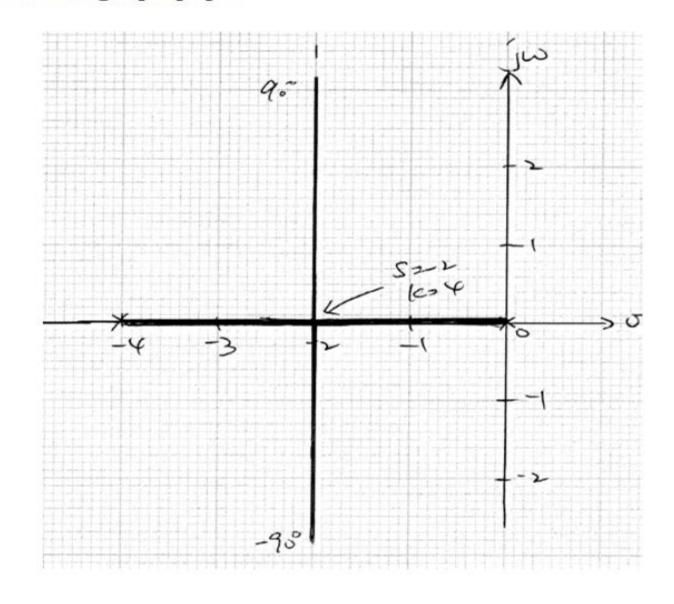
(a) The addition of a pole has the effect of pulling the root locus to the right, tending to lower the system's relative stability. The root locus plot is shown below.
