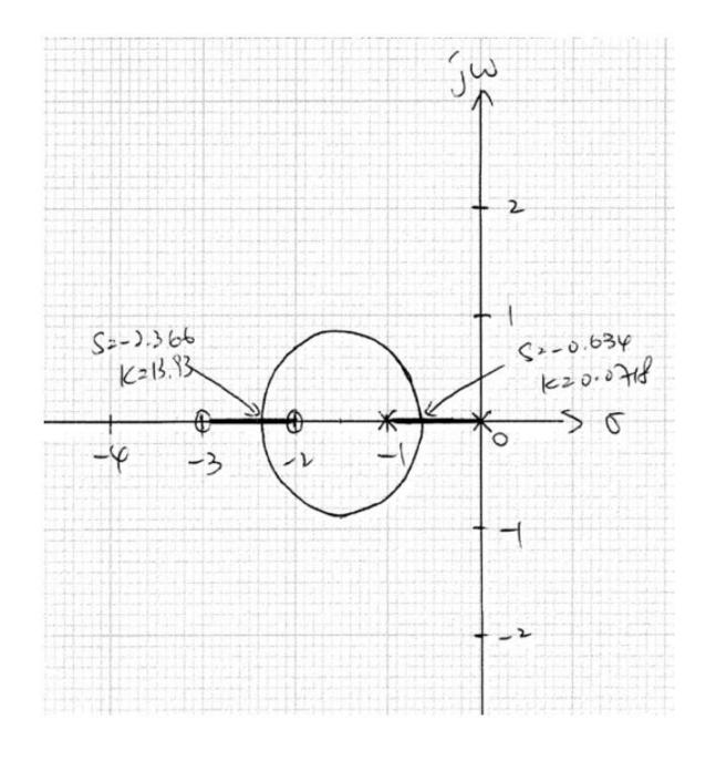
Sketch the root locus for the open-loop transfer function,
