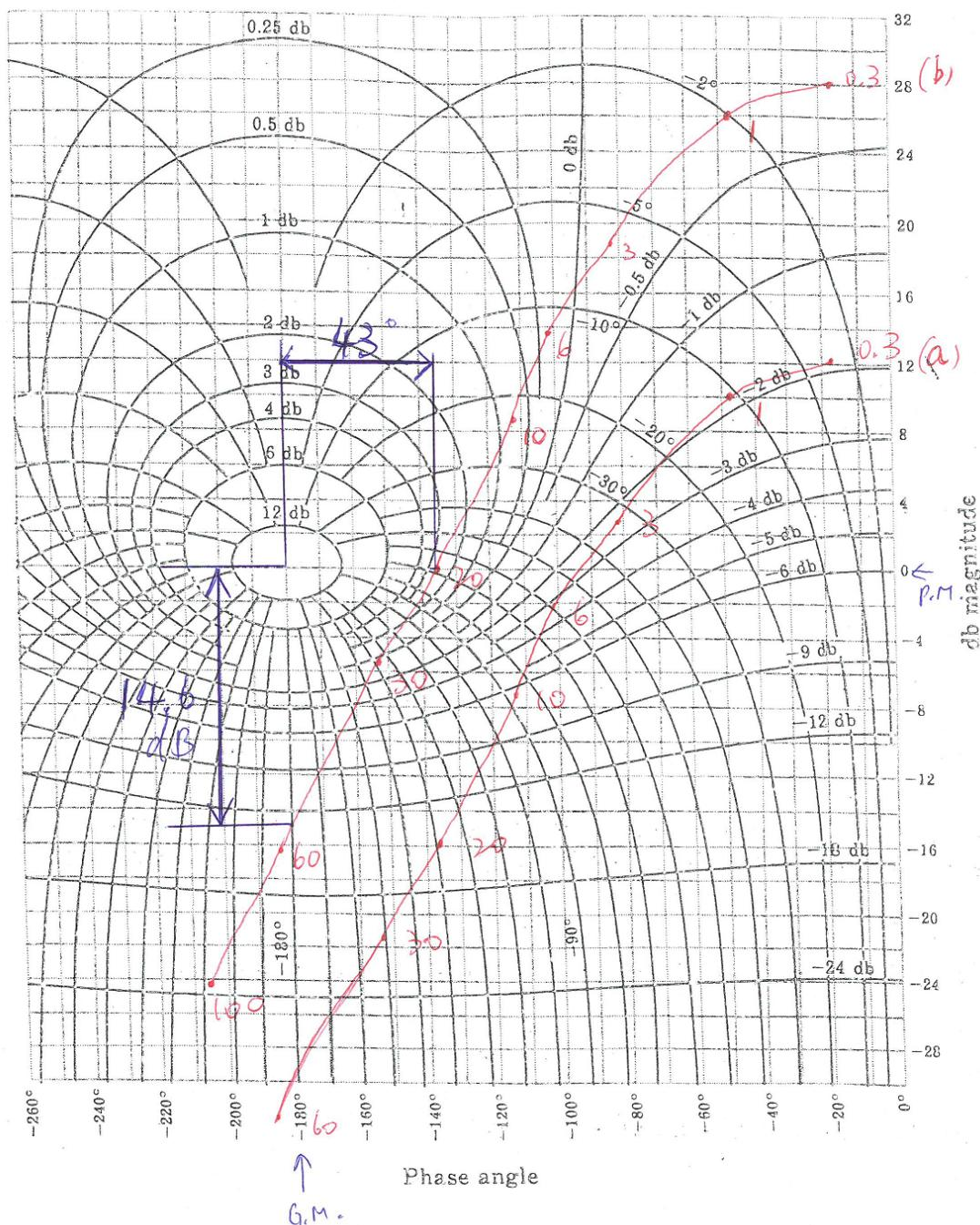
5. (b) (i) If the system gain is increased by 16 dB, the curve in the Nichols chart in part (a) & will shift up by 16 dB which is shown in the Nichols chart in part (a) as well.
