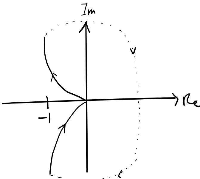
$$2. \quad (a) \quad |G(j\omega)H(j\omega)| = \frac{2}{\omega\sqrt{\omega^2 + 1}\sqrt{(2\omega)^2 + 1}}$$
