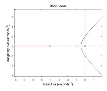
(b) The addition of zeros has the effect of pulling the root locus to the left, tending to make the system more stable. The root locus plot is shown below.
