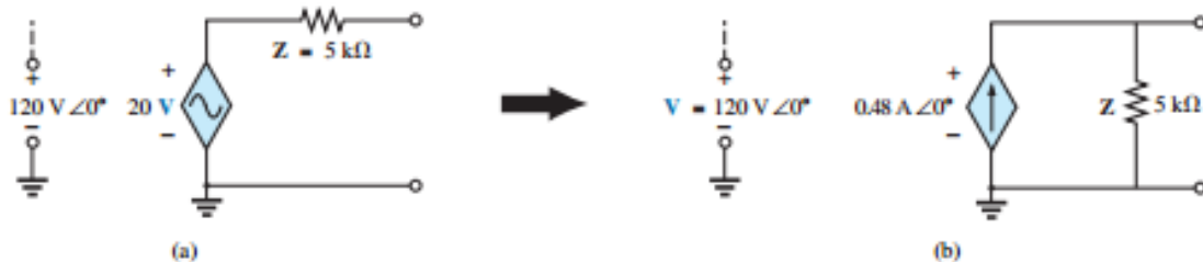
FIG. 18.8 Source conversion with a voltage-controlled voltage source.
