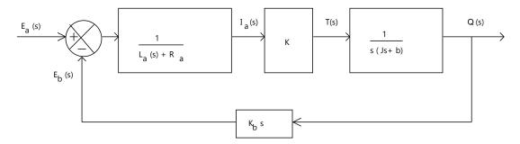
The DC motor in itself is a feedback system. The output velocity is directly related to the input voltage. The block diagram can be simplified into the following equation:
