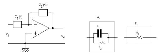
Since the circuit is similar to an inverter circuit, the transfer function is:
