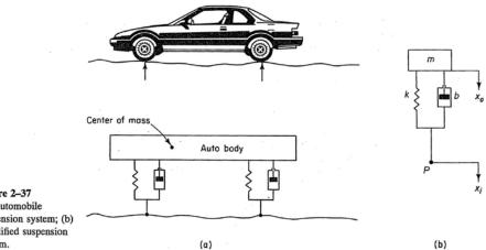
Figure 2-37 (a) Automobile suspension system; (b) simplified suspension system.
