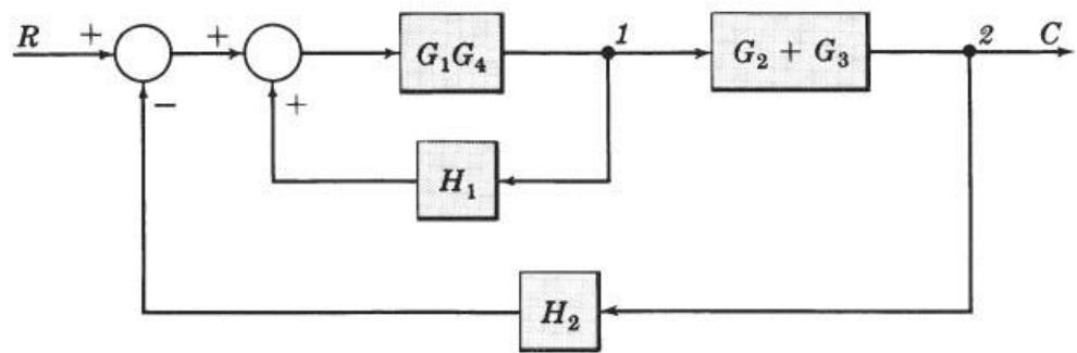
**EXAMPLE 7.10.** Let us reduce the block diagram of Example 7.9, isolating block  $H_1$ .
