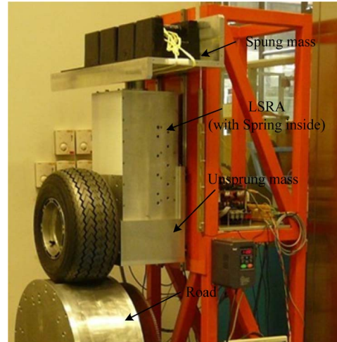
Fig. 5. Experimental setup of quarter-vehicle model.
