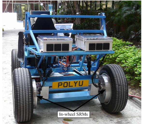
Fig. 19. EV prototype with two in-wheel SRM drives.
