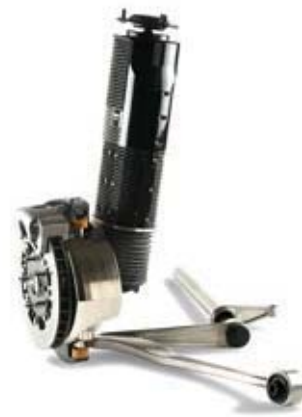
(a) Prototype of the electromagnetic active suspension developed by Bose Corporation
