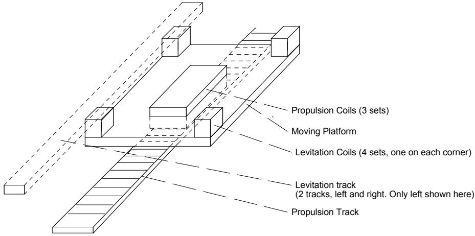
Figure 1 Layout of the Magnetic Levitated VR Linear Actuator
