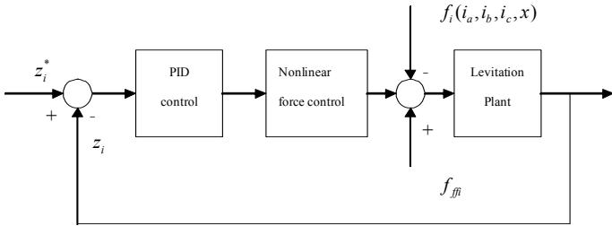
Figure 8. The control block diagram for the levitation coil – single coil.
