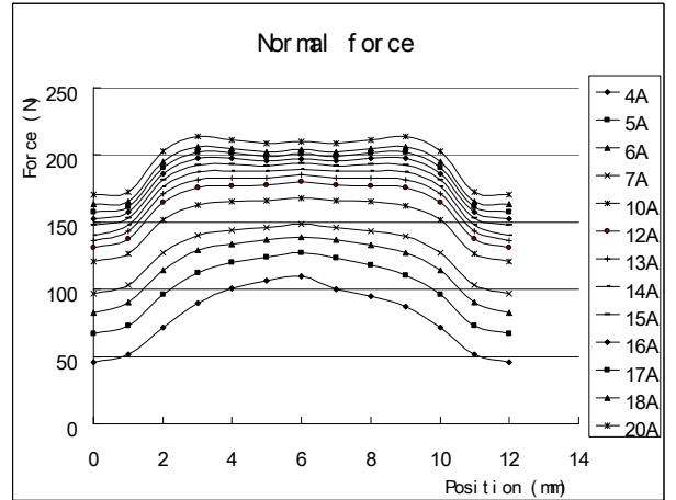
Figure 6. Normal force of the propulsion actuator.
