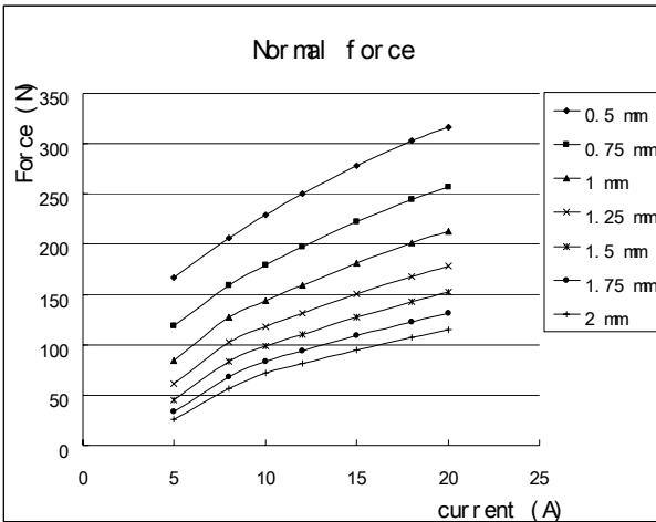
Figure 4. Normal forces of one levitation coil.
