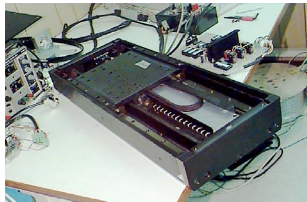
Fig. 1 A Linear Permanent Magnet Synchronous Motor
