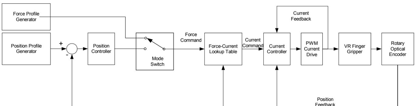
Fig. 8 An overall control block diagram
