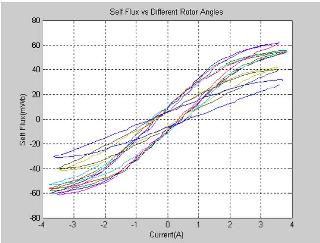
Fig. 3 Self Flux linkage versus different rotor positions
