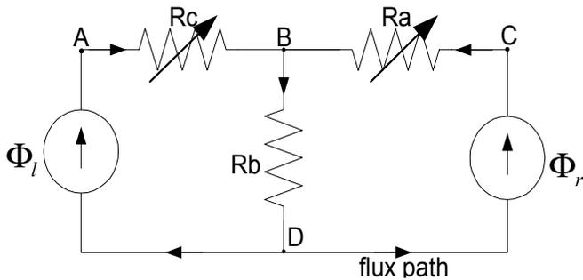
Fig. 6 Equivalent VR Gripper magnetic circuit representation
