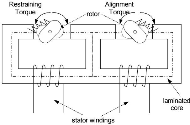
Fig. 2 Essential Parts of the VR Finger Gripper
