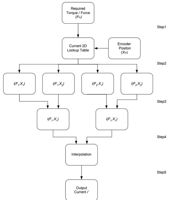
Fig. 9 Flowchart for Calculating  $i^*$
