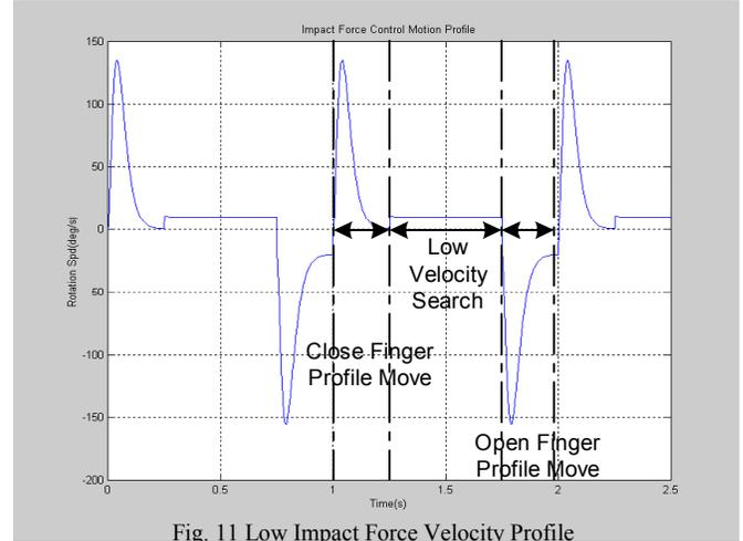
Fig. 11 Low Impact Force Velocity Profile
