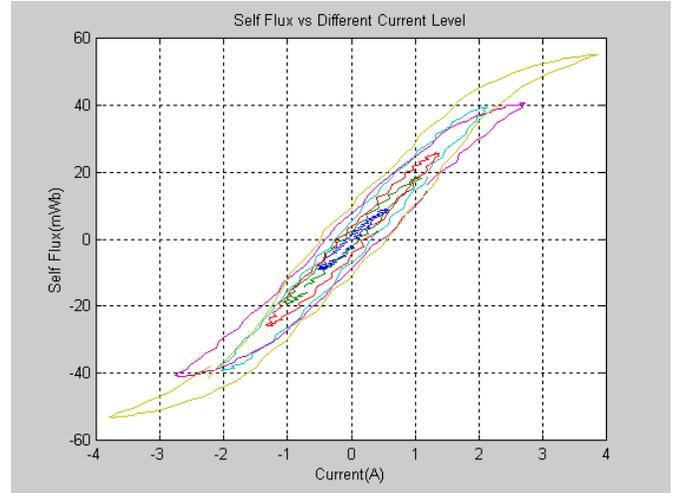
Figure 4. Self Flux linkage versus different current level
