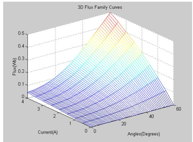
Fig. 5. 3D-Flux linkage profile of VR Gripper
