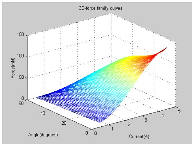
Fig. 7 3D Force profile of VR Gripper
