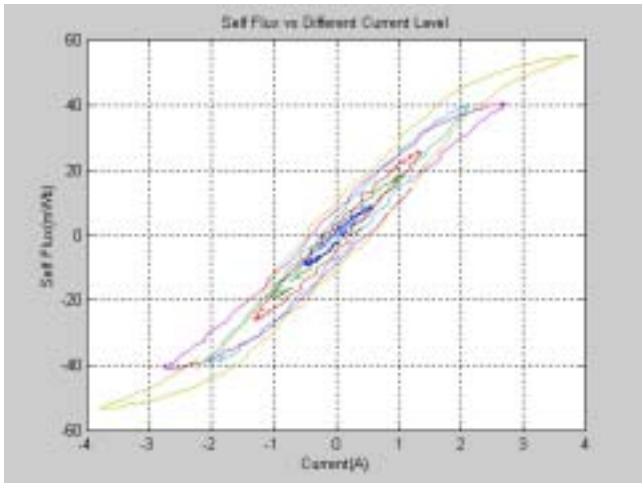
Fig. 5. Self Flux linkage versus different current level
